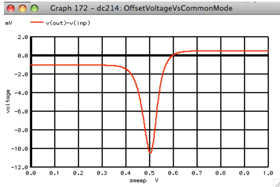
On a 1volt supply, both pnp and npns are off at 500mV.
