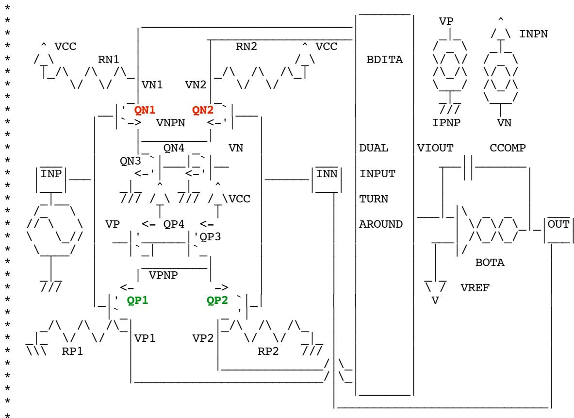
For the case of Bipolar transistors, this meant that two input stages need to be connected in parallel. Just doing so means most of the time both input stages are on and depending on which rail the inputs approach, one of the input stages will turn off.
