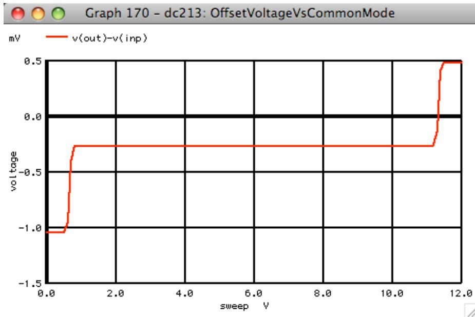
In this simulation, a 1mV mismatch was introduced to the input pnps and a +.5mV mismatch was introduced to the npns. So for most of the common mode input range, there is a partial offset cancelation. At zero volts the npns are off and the pnp's offset dominates. At 12Volts the npn's dominate.
