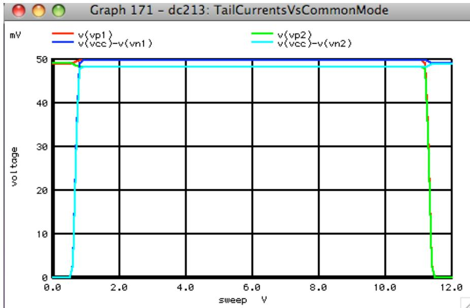
Another place to view things is the IR drop at the collector resistors for input transistors. If the resistors are small enough, the inputs can easily swing 200mV past both rails. This nodes later get fed into a dual input turn around circuit which converts the differential input signal from either input into a output current.
