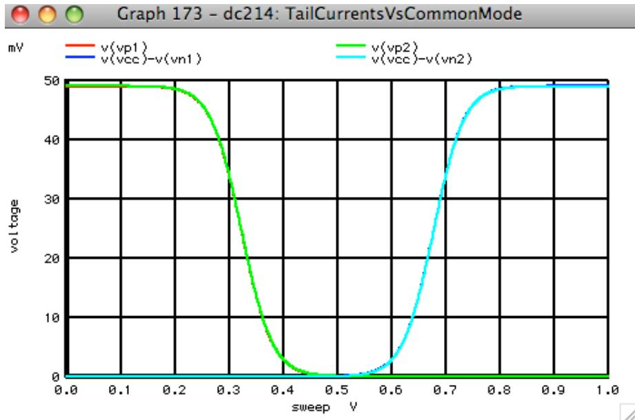
For a bipolar Rail To Rail Op Amp, this implies that there is a minimum supply voltage of two diodes and to sats in order that neither input stage is turned off.
