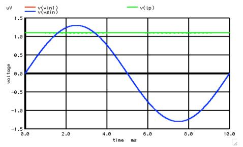
The chopper effectively passes the desired input signal through unchanged while it modulate all other undesirable signals up to the chopping frequency where they can be lowpass filtered out.
