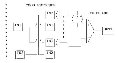
Chopping the input signal using switches is really just modulating or multiplexing a low frequency signal up to the chopping frequency. If the chopping frequency is high enough, the modulated input signal is well above the offset and 1/f noise of any amplifier which follows the chopping switches. This is the trick where signal gets placed where it can be distinguished from everything else.
