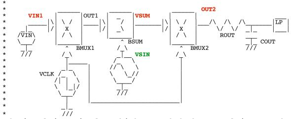
If signal is gained up high enough before applying to the second modulator, a standard four quad multiplier circuit will do the job.
