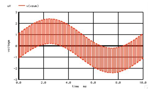
When this signal get remodulated by the same clock, the DC signal will return back to its original form. But the AC signal is now being modulated by the same chopping clock frequency.
