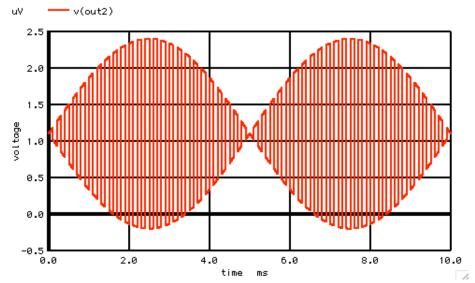
The desired 1.1uV VIN1 signal can be extracted by applying a low pass filter.
