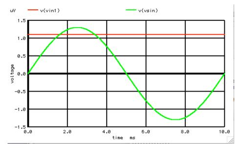
The sum of the modulated DC signal and the AC signal are shown below.
