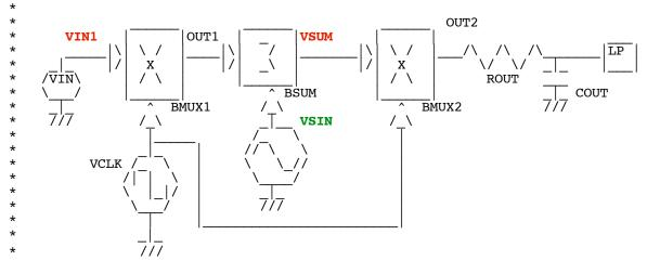
The simulation shows how this is done by applying a 1.1uV DC voltage in front of the input choppers and summing the output with a 100Hz sign wave to represent 1/f noise.
