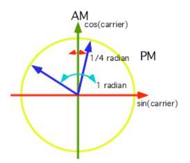
What if PM is generated by four Quad modulating a carrier to produce the right magnitude and phase? Start off doing a polar to rectangular conversion of a unity magnitude vector which has its angle being modulated by a 0.25radian sine wave. The Y direction represents the signal to be modulated by the cosine of the carrier. The X direction represents how the sinewave carrier will be modulated. The following Macspice simulation will do just that.
