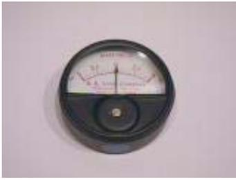
This is a meter my brother had purchased in order to insure there was no residual magnetic field left on some equipment. It would show polarity and magnitude. It was made by Anno Instruments in Indianapolis. It is very sensitive. The area at the bottom of the meter is placed near the magnetic field to be measured.
