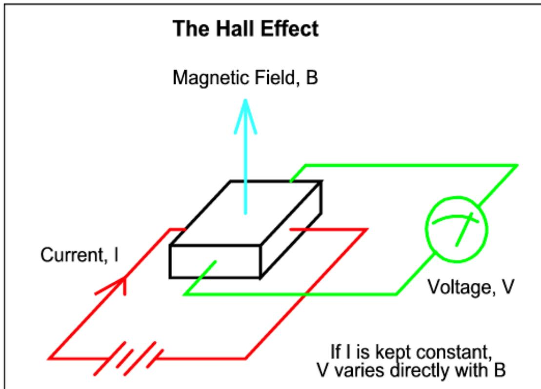
What can you do with a Hall-effect device? Build an electronic circuit which will amplify the voltage across the device and calibrate it so you can measure a voltage and translate that into a Gauss measurement. For such a unit, check out the page on building a [Gaussmeter](#).
