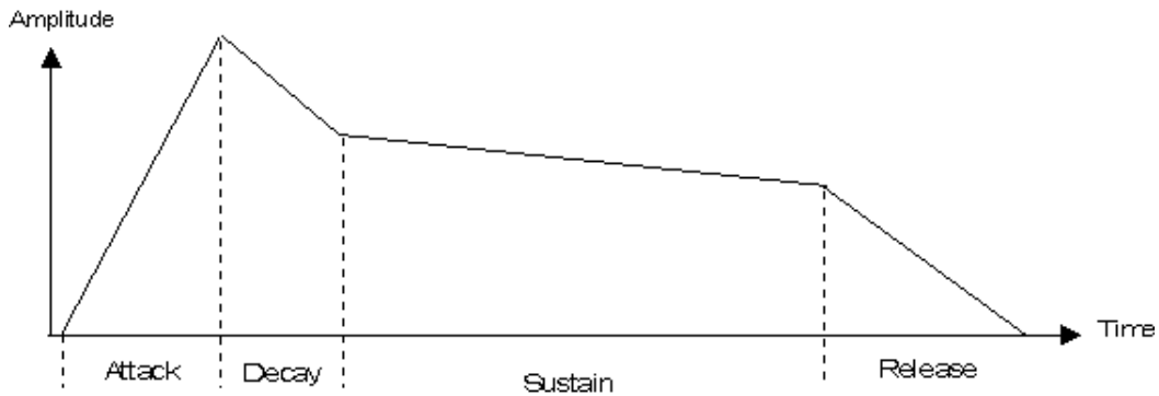
Figure 6: A Typical ADSR Amplitude Envelope
